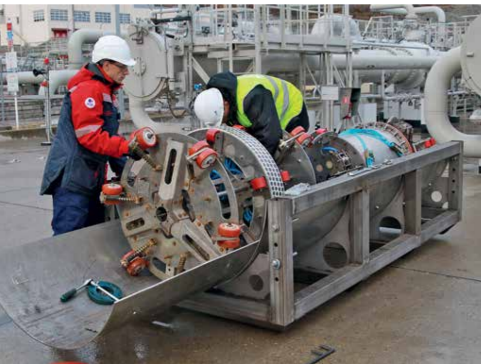
IN-PIPE FLAW DETECTOR (IN THE FOREGROUND)
