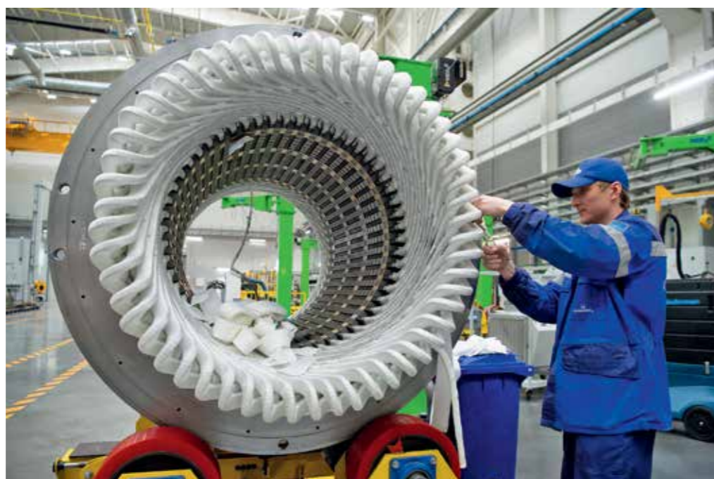
HIGH VOLTAGE MOTOR STATOR WINDING
