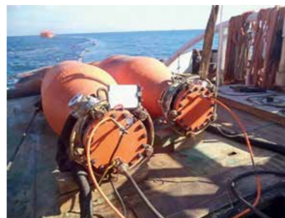
THE RAILING HOSES OF THE SPM FLOATING STRINGS ON BOARD THE MAINTENANCE TUGBOAT
